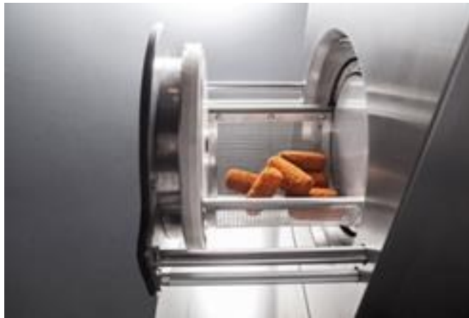
Abb. 4.2.5: Superheated steam Friteuse HiFri© (QBTEC BV, 2015)
